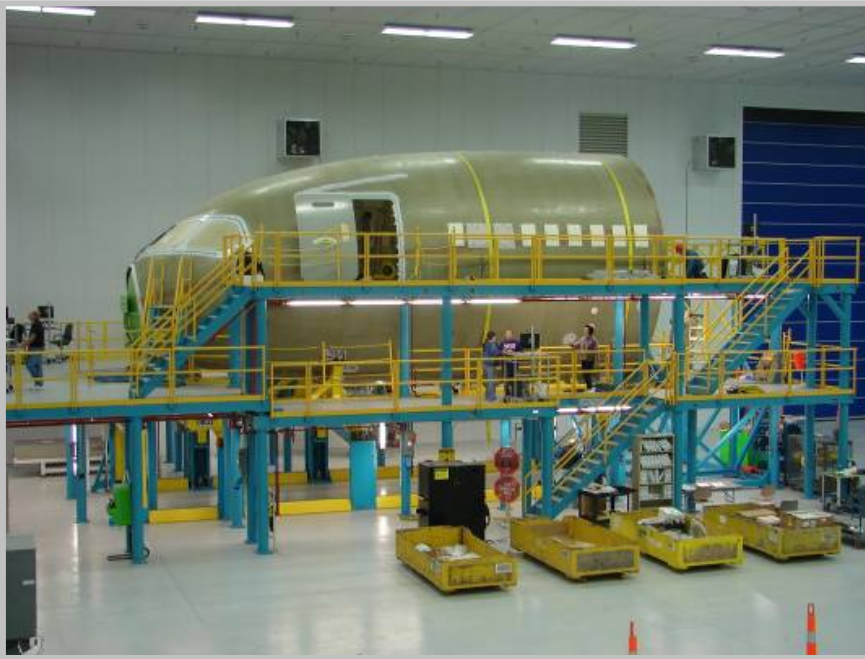
Line Unit 3 - Systems Installation
