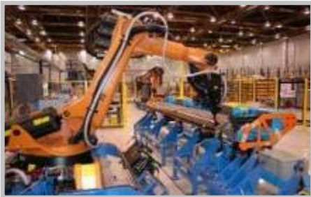
787 Slat Automated Robotic Drill
