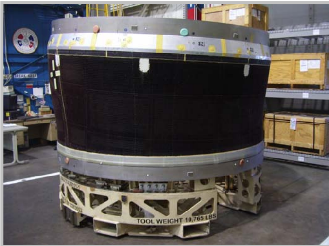
747-8 One Piece Inlet – Core Bonded To Inlet
