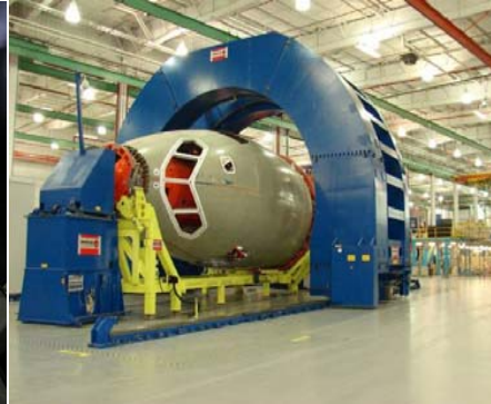
Cockpit Structure Installed
